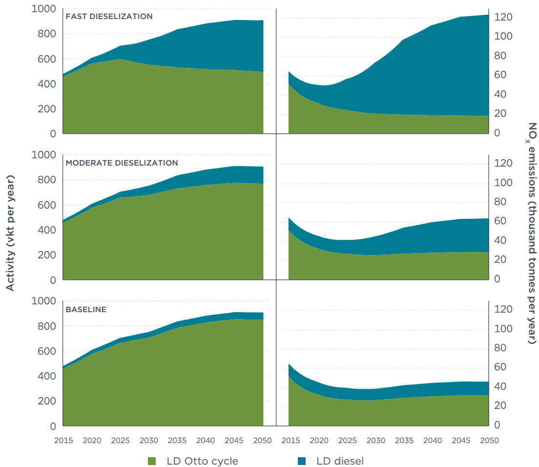
Figure 10. Projected LDV activity (left panels) and NO x emissions (right panels) separated according to engine type. LD Otto cycle and diesel contributions are shown for each scenario in green and blue, respectively.
